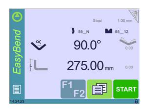
The EasyBend page is used for individual bends, for example when an external worker needs to interrupt production just to make a single bend (usually with the same tools).
