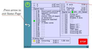
On the upper line, a cycle message may appear indicating the cycle phase the machine is executing
